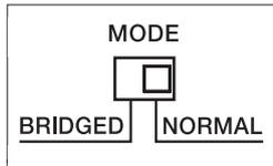
Switch for changing from normal (stereo) operation to bridged mode. In bridged mode the integrated power amplifiers operate in „push-pull“ operation. The output voltages of channel „A“ and channel „B“ are doubled and present at the BRIDGED OUT connector. Channels „A“ and „B“ work phase-shifted in push-pull operation and may not be used as loudspeaker outputs.
